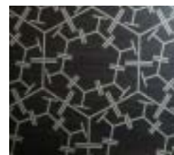
Fig.3 Outer Appearance of a dual band FSS for Wireless LAN (Close-up picture)
